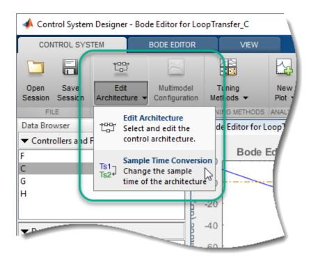
In the Sample Time Conversion dialog box, specify the **Sample time**, and select a **Conversion method** for each block in the control system. For more information on the available conversion methods, see Continuous-Discrete Conversion Methods. **Control System Designer** does not support the new least-squares vector fitting approach.
