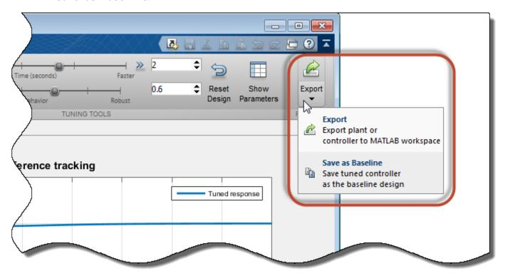
When you do so, the current Tuned response becomes the Baseline response. Further adjustment of the current design creates a new Tuned response line.
